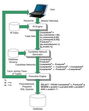
Figure 1: Architecture of our query processing system.
